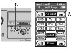
If it is necessary to adjust the output level of each channel, tap the CH Sel and Ch Level (PAGE6/8) on the remote control unit.
